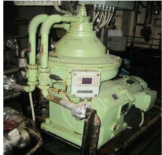
Gambar 2. Fuel Oil Purifier (Sumber: Dokumen Google)
