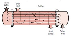
Figure 2. Shell and tube heat exchanger
