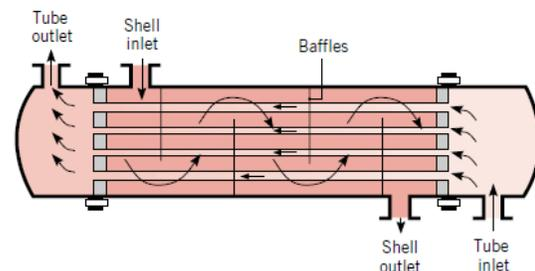
**Figure 2.** Shell and tube heat exchanger
