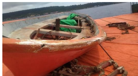
Figure 2. Condition of Damage to Lifeboat at KM. Forward 99
