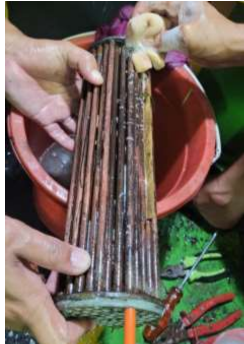
Gambar 1. lube oil Cooler Generator No 3
